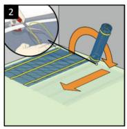
**Cut the mesh (not the cable)** Turn the mesh 180° and continue rolling
