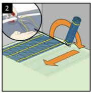
**Cut the mesh (not the cable)** Turn the mesh 180° and continue rolling
