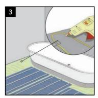
**Loose run for irregular areas** Remove the cable from the mesh, arrange and stick down
